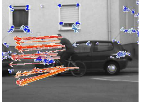
Fig. 4. Velocity estimation results for cyclist moving in front of parking cars. The arrows show the predicted position of the world point in 0.5s. The right image was taken 0.5s later allowing a comparison of the estimation from the left image. Blue encodes stationary points.
