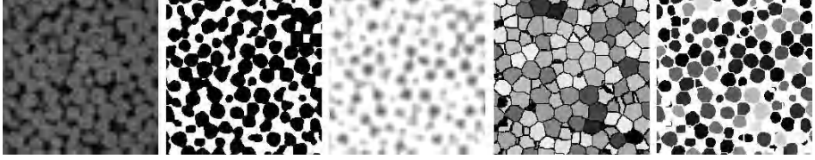
Fig. 2. Example for the segmentation processing chain, from left to right: Original image slice, binarization, Euclidean distance transformation (EDT) of the inverse binary image, watershed transformation of the inverse EDT image and labeled sinter balls.
